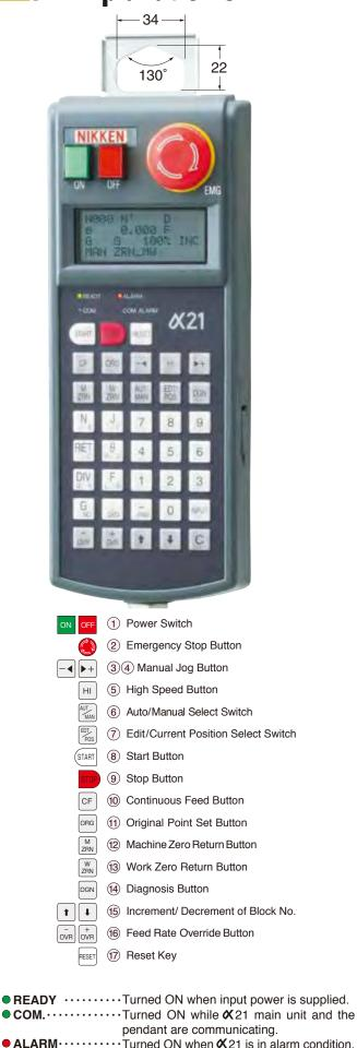
● ALARM ·········· Turned ON when **X**21 is in alarm condition. • COM . ALARM ····· Turned ON when communication time out error occurs between X21 main unit and the pendant.
