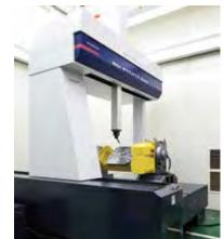
Accuracy measurement with large **3 Dimensional Measuring Machine**
