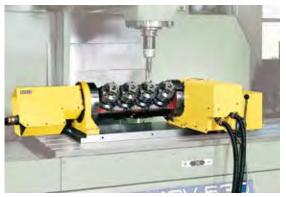
Tilting rotary table with Multi-Spindle
