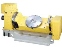
Built-in type 17 ports rotary joint is optional accessory. The position of the motor of the tilting axis table can be right or left side for the vertical M/C.
