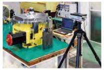
Indexing Accuracy Measurement by Laser
