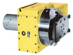
Rotary Joint is a rotating connector to supply air, hydraulic pressure or coolant liquid from outside to a fixture on a CNC rotary table. If liquid is supplied with ordinary hoses, twisting will happen on them by rotation of the table. However, rotary joints can solve this problem as it rotates in accordance with the table.
