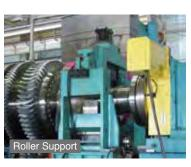
CNC1201 Indexing of the turbine shaft. Turbine shaft is supported and clamped by the roller support.
