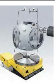
Configuration of the large rotary table on the horizontal M/C to machine a propeller hub of the windmill.
