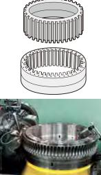
Hobbing of the gears with large module
